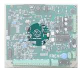
The FMF 2301, consists of a single measurement and output board, which vastly improves the reliability of the system. The interconnects are minimized and the accuracy is improved.
