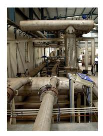
The Flow lab consists of two state of the art stainless steel rigs with the state of the art instrumentation, data acquisition and calibration software. The rig confirms to ISO-4185 standards and has been designed fabricated and commissioned 100% in-house.
